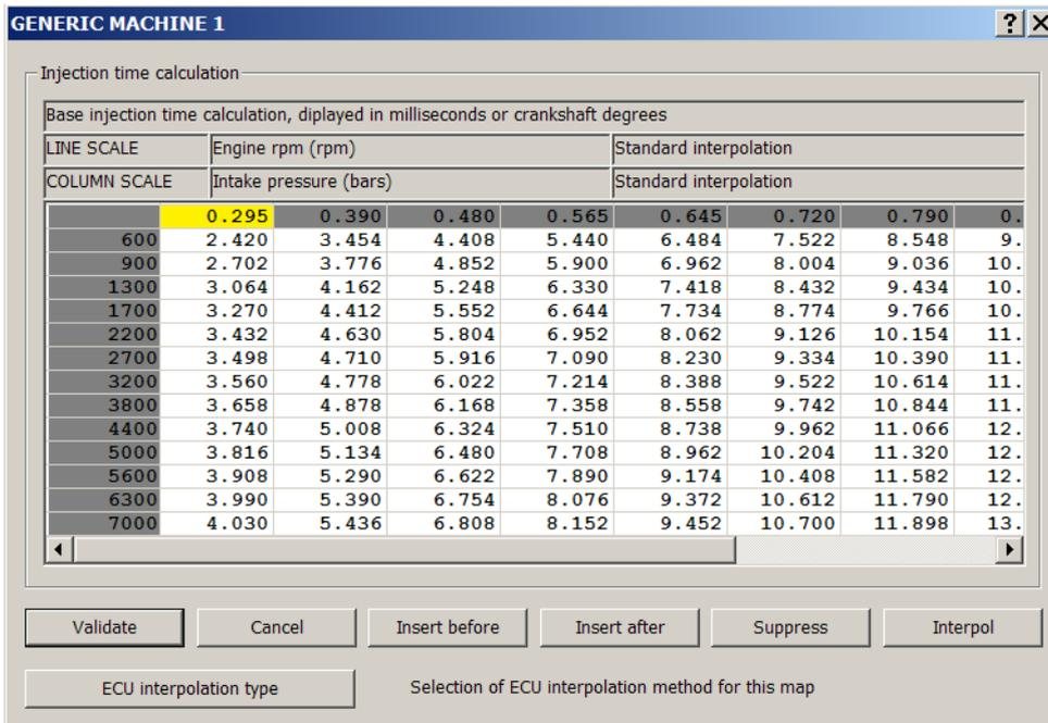
If you create new lines or columns, use the interpolate function to fill these lines or columns not to leave with null I.T. in the map (see user's manual of Winjall).
